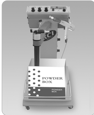
● KCI-206 : Hopperless type (Vibrating Plate instead of Powder Container)
